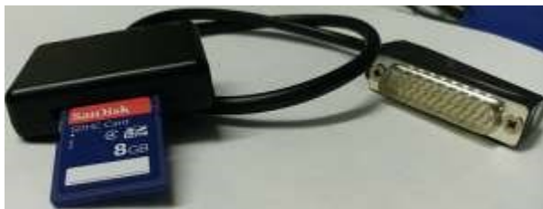
QL-SD, parallel port prototype, with 8GB SDHC card
